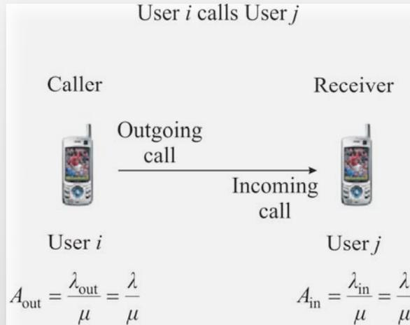
A traffic intensity of 1 **erlang** implies that a channel will be occupied for 60 minutes during an one-hour period.
